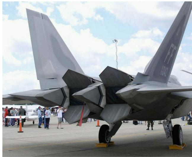
**Figure 2. Thrust vectoring nozzles on the F-22 Raptor**
